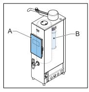
The user selects a desired quantity of beverage on the control panel (A). The continuous flow heater (B) inside the tower heats the corresponding quantity of water.
