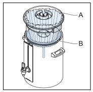
The basket filter (A), a paper filter, and a pre-loaded coffee product receive the hot water. The filtered coffee then flows through the coffee blender (B) into the container.
