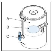
The container (A) keeps the hot beverage ready for consumption. The container has a tap (C) to serve the beverage. The CNe model container has an electric element (B) to keep the beverage heated.
