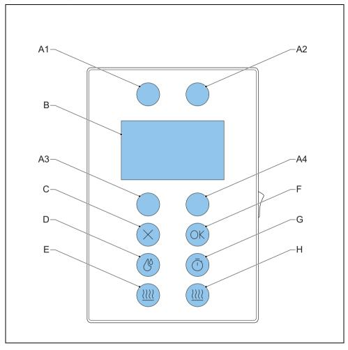
A: (A1, A2, A3, A4) Selection buttons. Also use A2 to go to the operator menu. Refer to section 2.5.1 B: Display
