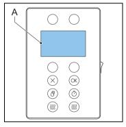
The display (A) shows technical malfunctions with error codes. The display also provides additional user information or warnings.
