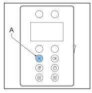
The stop button (A) stops the brewing process. The machine is still charged after the brewing process is stopped. Unplug the machine to make sure that the machine is entirely uncharged.
