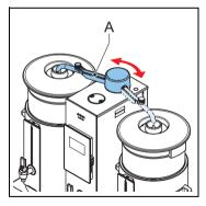
The swivel arm (A) directs hot water from the continuous flow heater into the top of a distributor lid.
