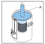
The tea filling pipe and filter unit (A) receive the hot water and combine it with a pre-loaded tea product inside the container.
