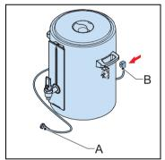
The container model CNe is connected to the electric socket with an electric cable which is plugged into the container (B) and the socket (A).
