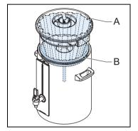
The basket filter (A), a paper filter, and a pre-loaded coffee product receive the hot water. The filtered coffee then flows through the coffee blender (B) into the container.
