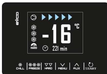
On completion of the blast chilling cycle, when the needle probe has reached the right temperature or the time period is finished, the buzzer sounds and the conservation phase begins. If the temperature controlled cycle is not completed in the allotted time, the problem will be notified by displaying an alarm message.
