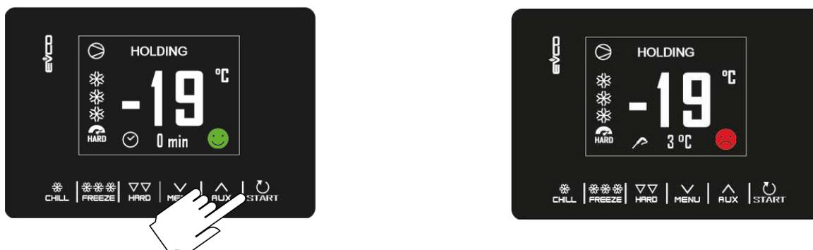
The conservation phase is not timed and is only terminated when the "Start" key is pressed for 2 seconds.
