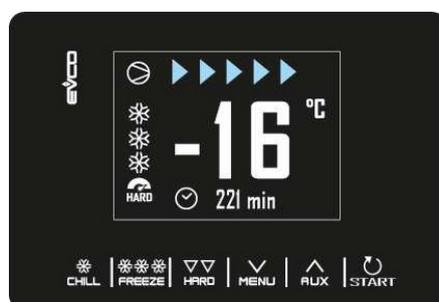
On completion of the blast freezing cycle, when the needle probe has reached the right temperature or the time period is finished, the buzzer sounds and the conservation phase begins. If the temperature controlled cycle is not completed in the allotted time, the problem will be notified by displaying an alarm message.
