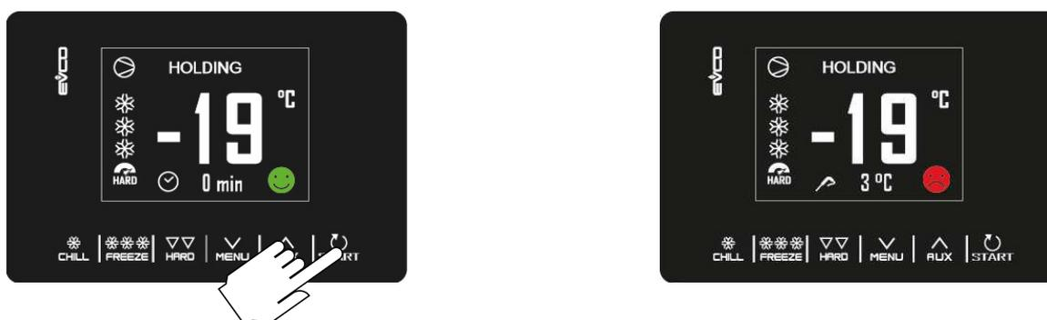
The conservation phase is not timed and is only terminated when the "Start" key is pressed for 2 seconds. Defrosting is always enabled during a conservation phase.
