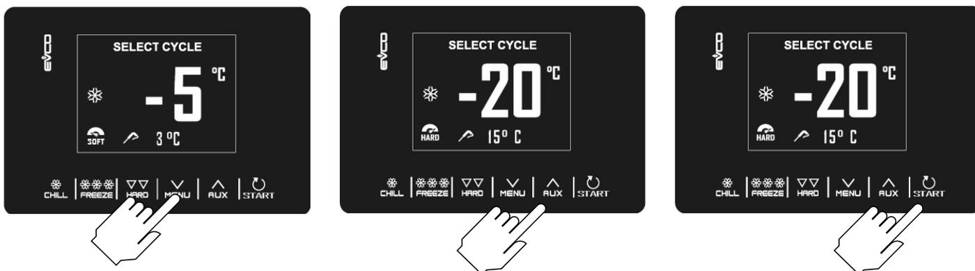
The selected cycle will offset either the pre-loaded settings for that cycle, or the settings of the last cycled carried out. By pressing "Aux" "Menu" it will be possible to quickly change the value of an individual data (set by parameter r35) within the permitted ranges. Once the change has been made press "Start" to carry out the cycle.
