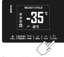
The selected cycle will offet either the pre-loaded settings for that cycle, or the settings of the last cycled carried out. By pressing "Aux" "Menu" it will be possible to quickly change the value of an individual data (set by parameter r35) within the permitted ranges. Once the change has been made press "Start" to carry out the cycle.
