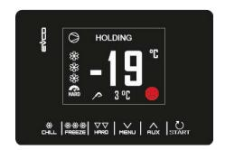
The conservation phase is not timed and is only terminated when the "Start" key is pressed for 2 seconds. Defrosting is always enabled during a conservation phase.
