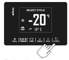
The selected cycle will offet either the pre-loaded settings for that cycle, or the settings of the last cycled carried out. By pressing "Aux" "Menu" it will be possible to quickly change the value of an individual data (set by parameter r35) within the permitted ranges. Once the change has been made press "Start" to carry out the cycle.
