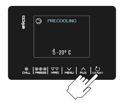
Once the required cabinet setpoint has been reached, the buzzer sounds and the cycle continues and maintains the cabinet temperature achieved until the "Start" key is pressed for 2 seconds or until a blast chilling/blast freezing cycle starts up.
