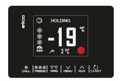
The conservation phase is not timed and is only terminated when the "Start" key is pressed for 2 seconds.
