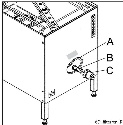
*Removing/fitting the filter*
