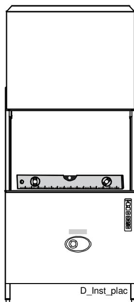
*Check using a spirit level that the machine is standing level*
