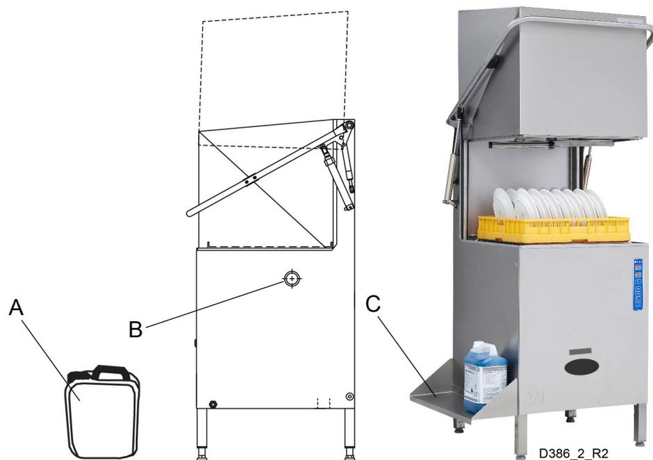
*The detergent (A) is positioned below the plugged connection for the detergent hose (B).*
