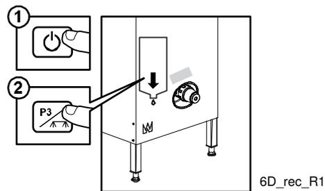
Note that emptying is necessary when you want to unscrew and clean the filter, because otherwise the water from the tank will spill out onto the floor.
