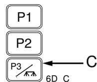
*The programme button "P3" (C) is used to start the cleaning programme and empty the tank for the recirculating rinse*
