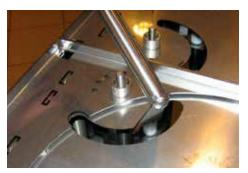
Slide the adjustment rods (4 pcs/cylinder) in place. You do not need to remove the cylinder from the appliance..
