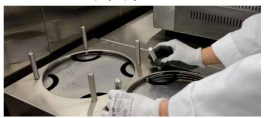
Remove the rods by screwing them counter-clockwise
