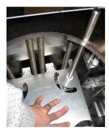
To access the springs, press an empty cylinder with your hand. Remove the attached spare spring. There is a hole in the dish platform for reserve springs to keep them in place.
