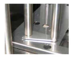
Lift the rod and turn it into the position desired. There are guide studs at the upper and lower end of the adjustment rod to ensure the correct location of the rod.
