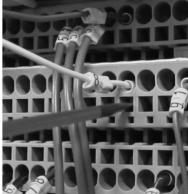
Connect the wiring for photocell B61 and B62 to the green contact J44 on computer card A1.
