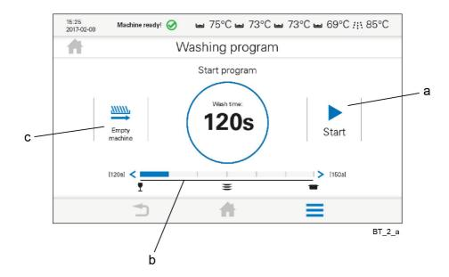
The contact time is the total period during which the load is washed while being transported through the various washing zones. There are six different times that can be selected.
