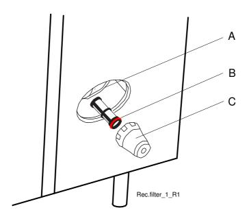
Removing/fitting the filter
