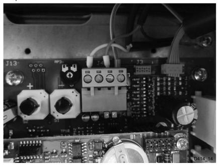
• Connect the temperature sensor to the terminal box in accordance with the machine's wiring diagram.
