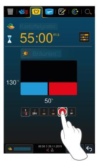
If you have started an intelligent cooking path, the display changes to the cockpit after a short time. All cooking steps that the intelligent cooking path processes are displayed here one after the other. The active cooking step is highlighted. The cooking steps that will take place in the future are greyed out. When the cooking step is completed, the next cooking step is automatically displayed.
