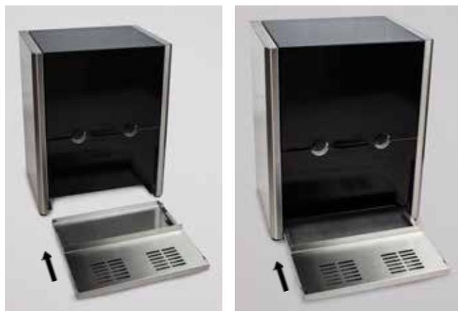
Push the drip tray assembly into the appliance as far as it will go. Only the perforation of the grill plate remains visible from the drip tray. The drip tray cannot be inserted if it is installed the wrong way round.
